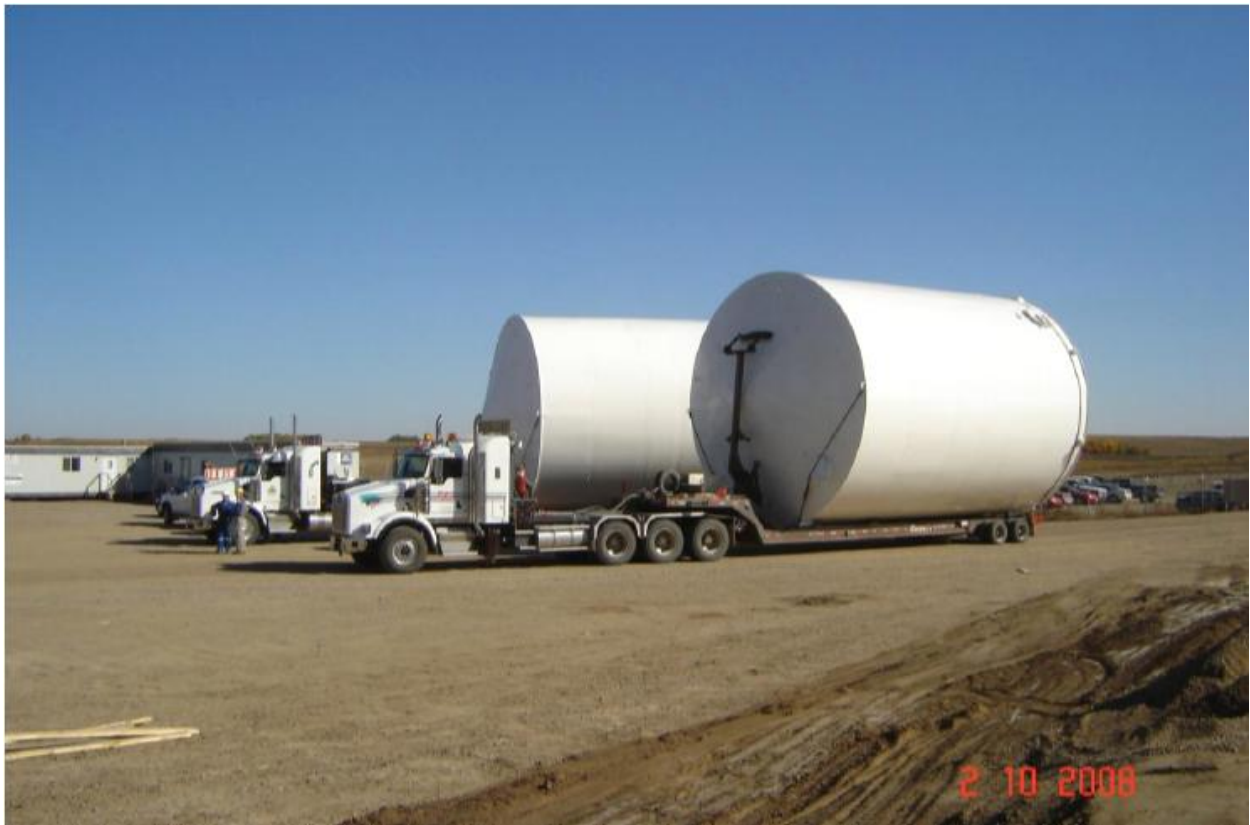
375,000 litre Ethanol Storage Tanks
